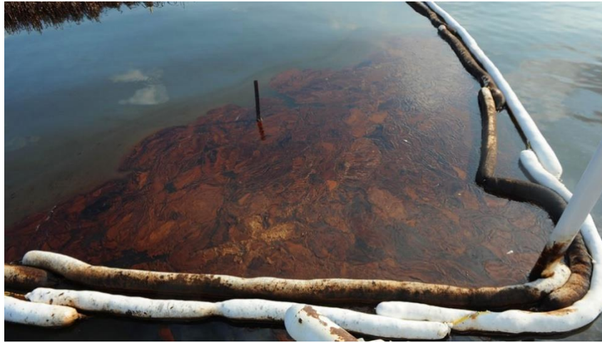
Figura 13. Barreras sorbentes. Adaptado de Complete Environmental Products (2020). Oil Only Absorbent Boom . Recuperado de http://www.cepsorbents.com/booms .
