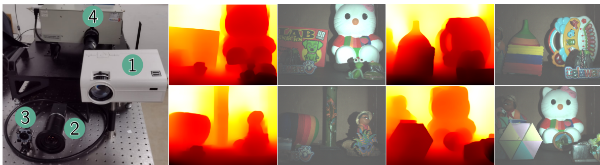
Figure 31. (left) Optical system used to acquire our own spectral-depth dataset using spectral scanning and structured light. The light projector (1) emits a collimated beam of structured light patterns that is captured by the camera (2). The tunable light source (4) emits selective wavelengths to travel through an optical fiber (3) to illuminate the scene which is also captured with camera (2). (right) A few samples of the acquired dataset.
