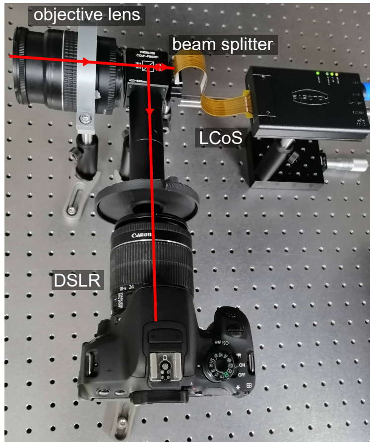
Figure 16. A photograph of the optical setup used in our compressive light field imaging experiments. The light path is shown in red and the various components are labeled.
