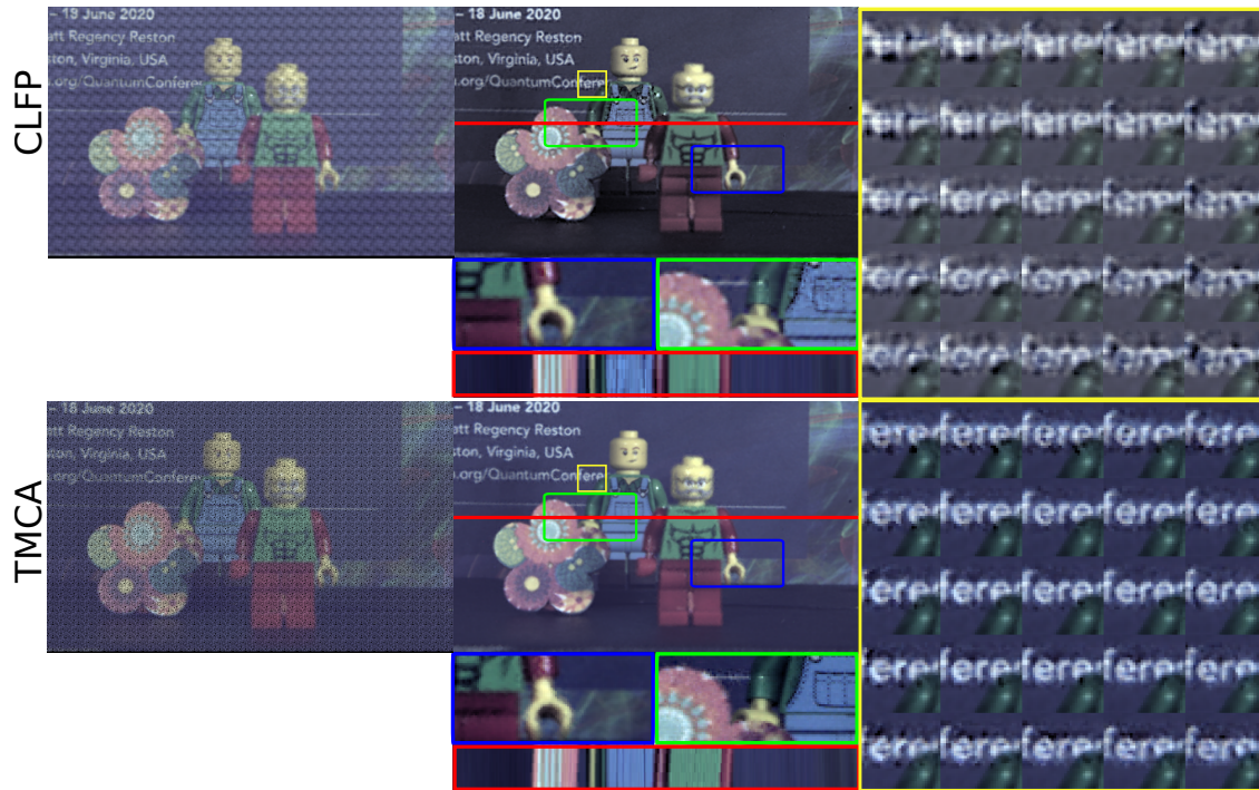
Figure 17. Real captures of coded snapshots for light fields comparing CLFP (Marwah et al., 2013) and the proposed TMCA with their reconstructions.
