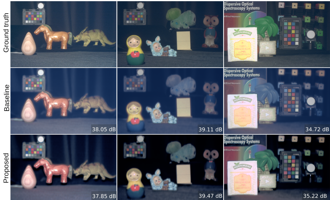
Figure 27. Comparison of the recovered spectral images, mapped to RGB, using our proposed TMCA method and the competitive baseline Baek et al. (2021). Visually, the colors of the proposed approach better resemble the ground truth, demonstrating a better spectral estimation. The PSNR between the recovered and the ground truth images is reported in the lower-right corner of each inset.
