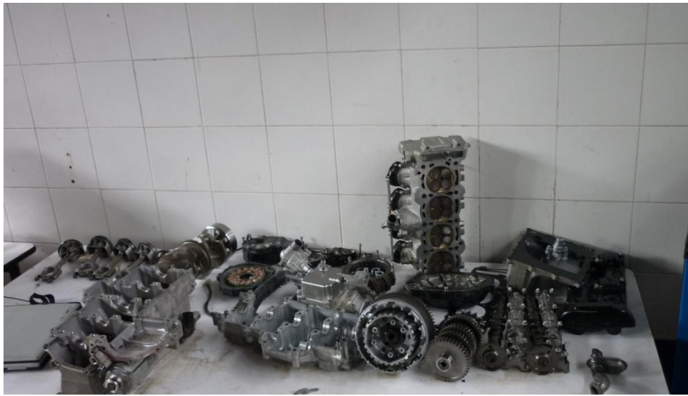
Figura 42.Despiece motor Gsxr 1000 K9 FORSSA
