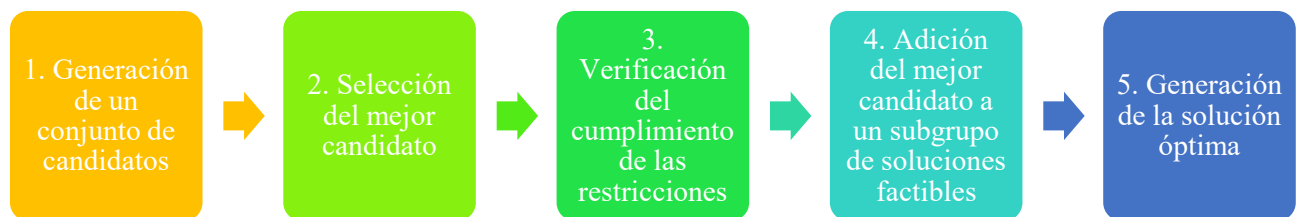
Figura 10. Etapas del algoritmo voraz. Adaptado de Shao, W., Pi, D., & Shao, Z. (2017). Optimization of makespan for the distributed no-wait flowshop scheduling problem with iterated greedy algorithms. Knowledge-Based Systems , 137, 163–181. https://doi.org/10.1016/j.knosys.2017.09.026
