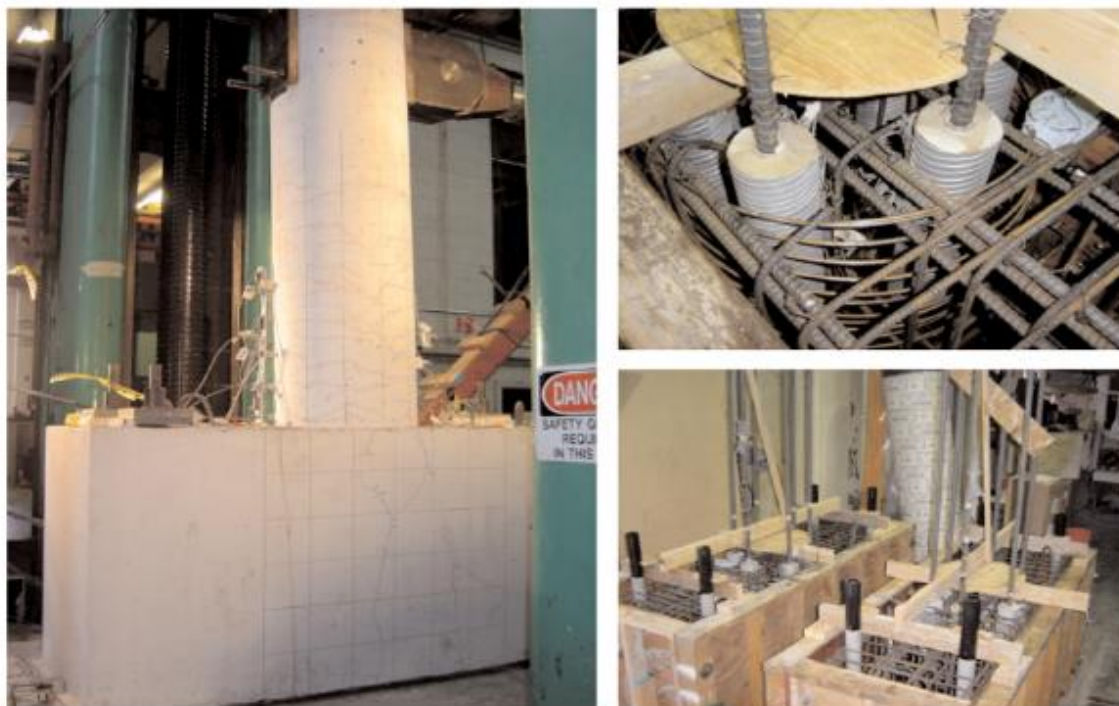
Figura 5. Construcción del modelo de estudio en la universidad de Washington. Adaptado de: Bijan Khaleghi. (2010). Washinton State Departamente of Transportation Plan for Accelerated Bridge Construction. Transportation Research Record: Journal of the Transportation Reach Board
