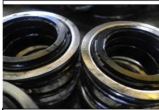
Mechanical seals were in good condition
