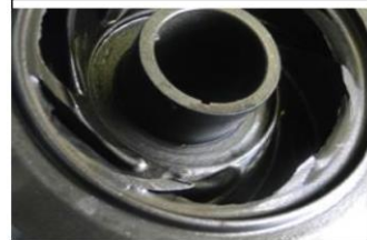
Impellers presented severe wear in vanes and skirt
