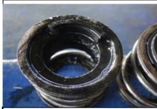
Part of lower mechanical seal was missed
