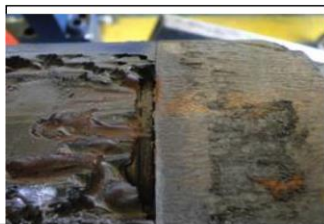
Motor's housing and base surface were found with corrosion
