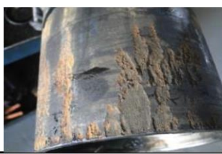
Housings surface presented corrosion
