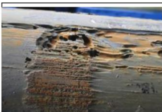
Motor's housing and base surface were found with corrosion
