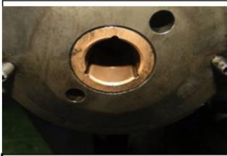
Base's bushing was ok
