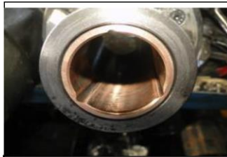
Base's bushing was ok
