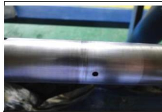
Shaft presented visual marks at bushing location
