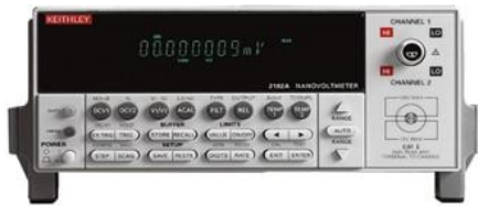
Figura 22. Nanovoltímetro 2182A. Adaptado de Keithley Instruments, I. (2004). Model 2182 and 2182a nanovoltmeter. User's Manual, 2–5
