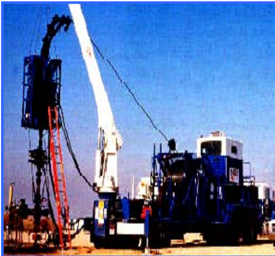
Figura 23. Unidad de Coiled Tubing.
