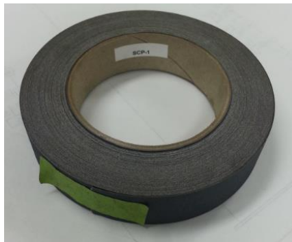
Figura 88. Lija 200-grit silicon carbide
