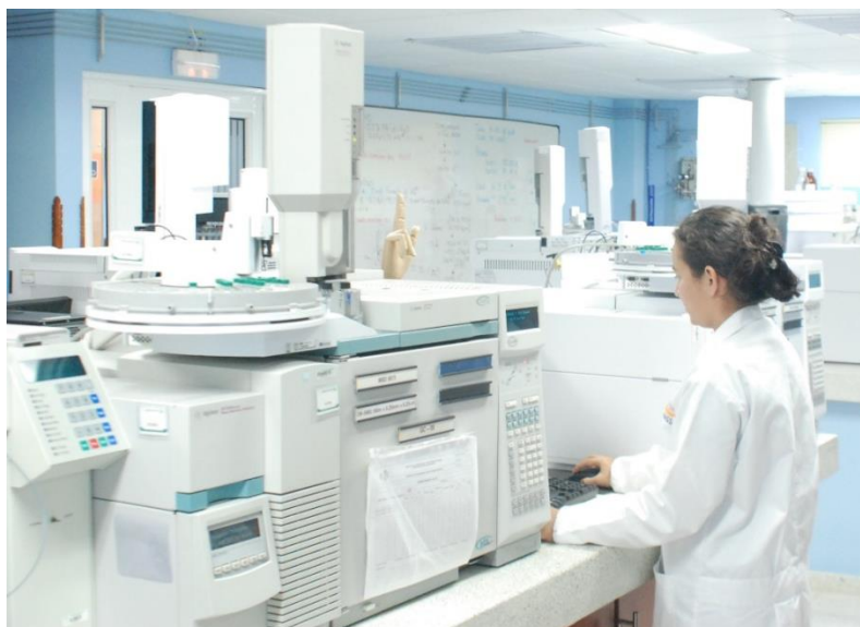
Figura 9. Agilent Technologies 6890A . Laboratorio instrumental CROM-MASS, UIS.
