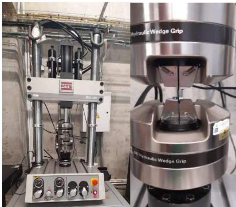
Figura 15.(a) Mechanical Testing Systems (MTS) , (b) Montaje de la probeta
