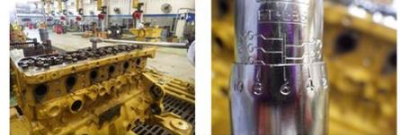
Picture 7. Cylinder head bolts check.
