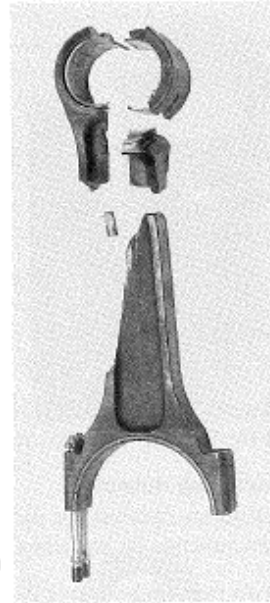
Fig. 6.138 Connecting rod fatigue failure.
