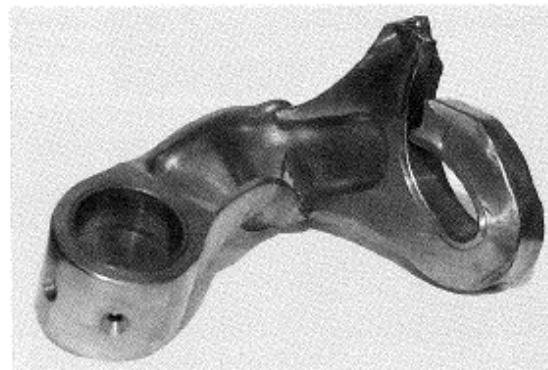
Fig. 6.150 Connecting rod failure as a result of hydraulic lock.
