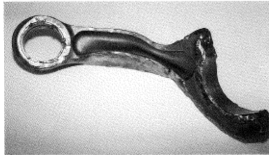
Fig. 6.149 Connecting rod failure as a result of connecting rod bolt fracture.
