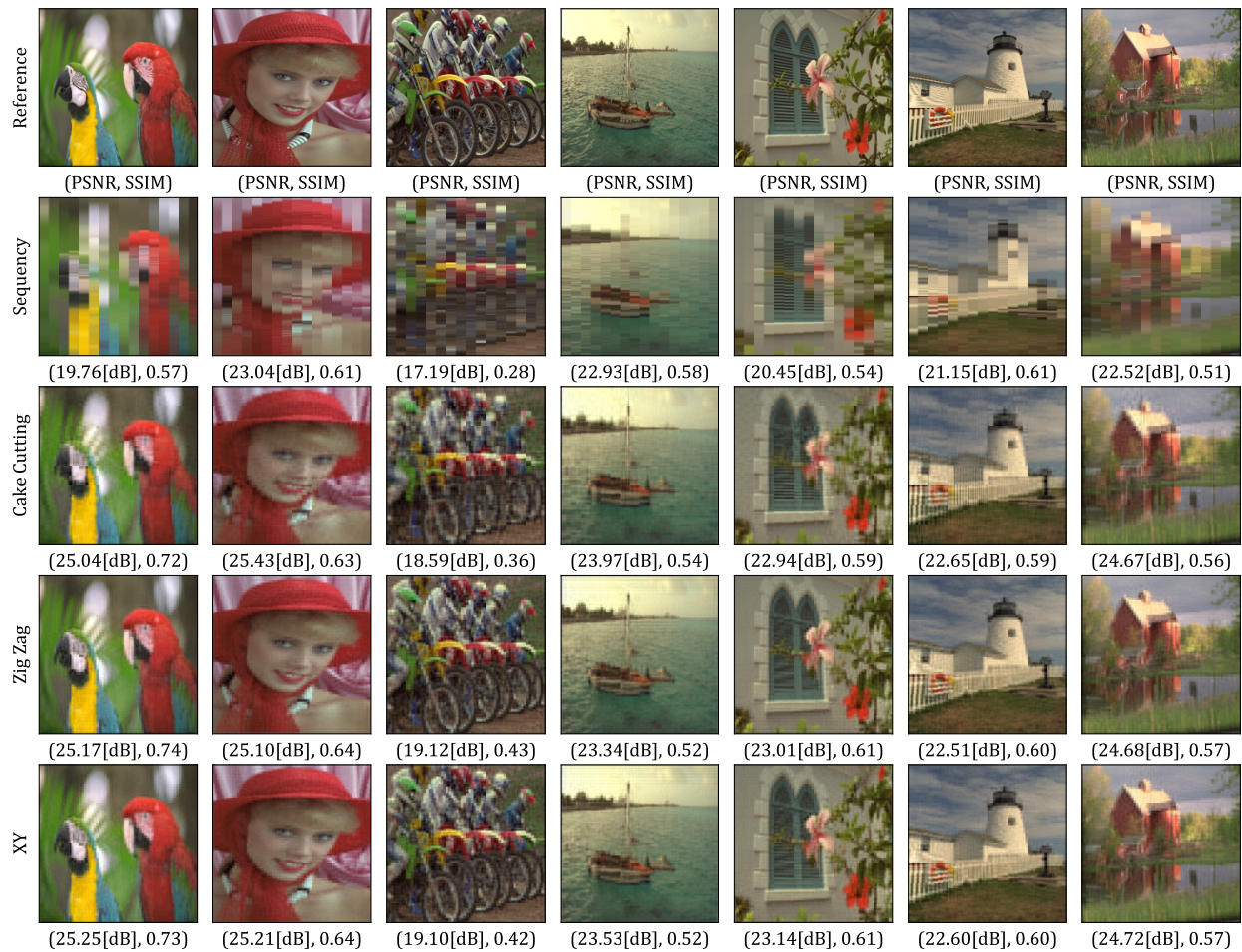
Figure 1. Effect of Hadamard ordering on Kodak images. The ideal Hadamard ordering technique (Sequency, Cake Cutting, Zig Zag, XY) that maintains the most significant spatial information and image quality differs depending on the specific scene.
