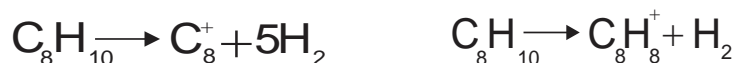
Figura 15. Mecanismos de deshidrogenación completa e incompleta del Xileno. Adaptado de Berg, C., Schindler, T., Lammers, A., Niedner-Schatteburg, G., & Bondybey, V. E. (1995). Dehydrogenation of Xylene Isomers on Niobium Cluster Cations Nbn+ (n= 2-26). The Journal of Physical Chemistry , 99(42), 15497-15501.
