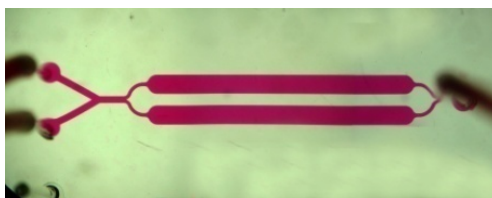
Figure 15. Design of simple micro-channel device used in our preliminary Biofilm experiments.
