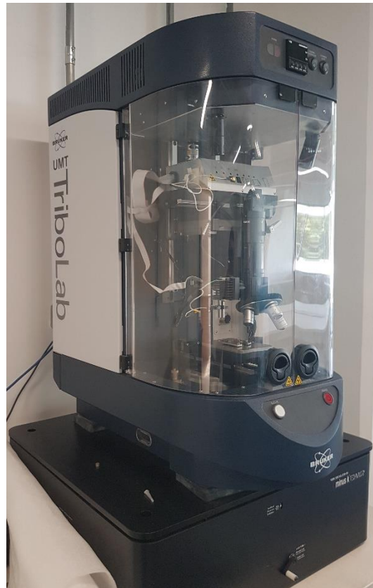
Figura 11. Tribómetro BRUKER UMT (Universal Mechanical Tester) Tribolab.
