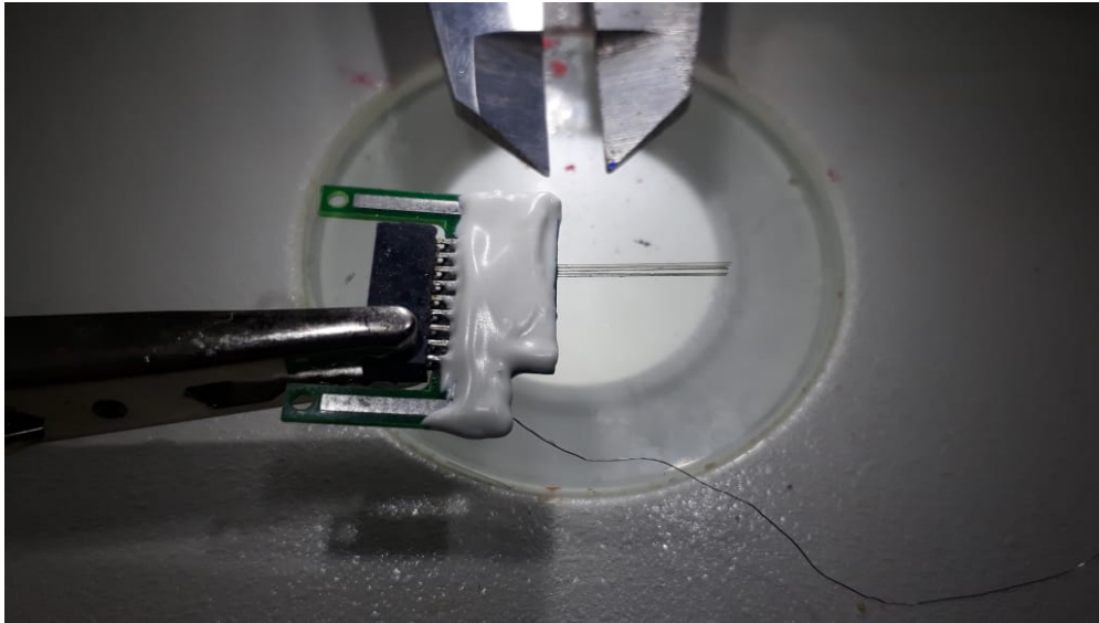
Figure 13. Electrodes matrix. Matrix with 8 50mm tungsten electrodes ready for recording, a common ground (GND), a reference for the channels (ref_elec) and a resin coating to fix all the components to their respective place.
