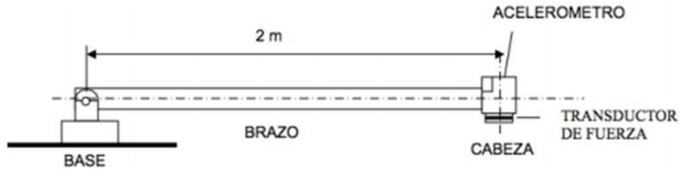
*Figura 31.* Configuración del Martillo de impacto vista longitudinal. Adaptado de Green, M. F. (1995, February). Modal test methods for bridges: a review. In PROCEEDINGS-SPIE THE INTERNATIONAL SOCIETY FOR OPTICAL ENGINEERING (pp. 552-552). SPIE INTERNATIONAL SOCIETY FOR OPTICAL.
