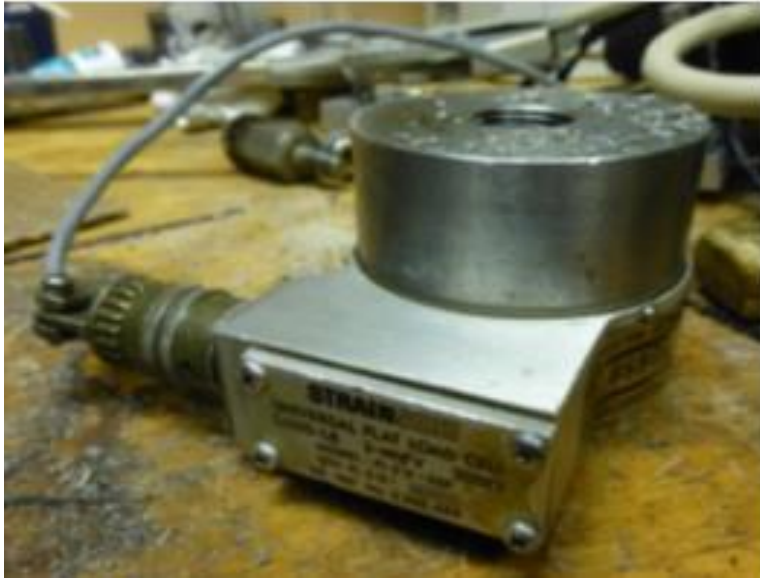
Figura 41. Celda de Carga StrainSert FL5U-2SPKT. Adaptado de Northmore. A. (sf). Canadian Solar Road Panel Design: A Structural and Environmental Analysis
