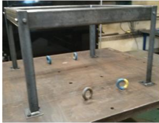
Figura 38. Plataforma de prueba estructural. Adaptado de Northmore. A. (sf). Canadian Solar Road Panel Design: A Structural and Environmental Analysis
