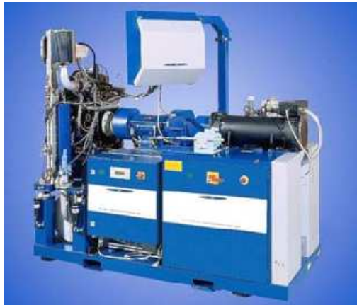
Figura 23. AVL 570 Single Cylinder Compact Test Bed
