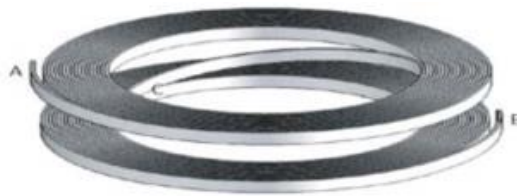
Figura 30. Configuración solenoidal. Adaptado de Zhu, J., Zhang, H., Yuan, W., Zhang, M., & Lai, X. (2013). Design and cost estimation of superconducting magnetic energy storage (SMES) systems for power grids. Vancouver: IEEE.
