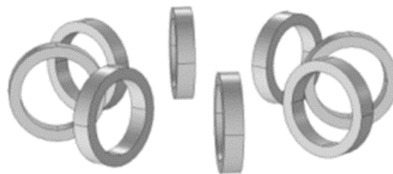
Figura 29. Configuración toroidal. Adaptado de Zhu, J., Zhang, H., Yuan, W., Zhang, M., & Lai, X. (2013). Design and cost estimation of superconducting magnetic energy storage (SMES) systems for power grids. Vancouver: IEEE.
