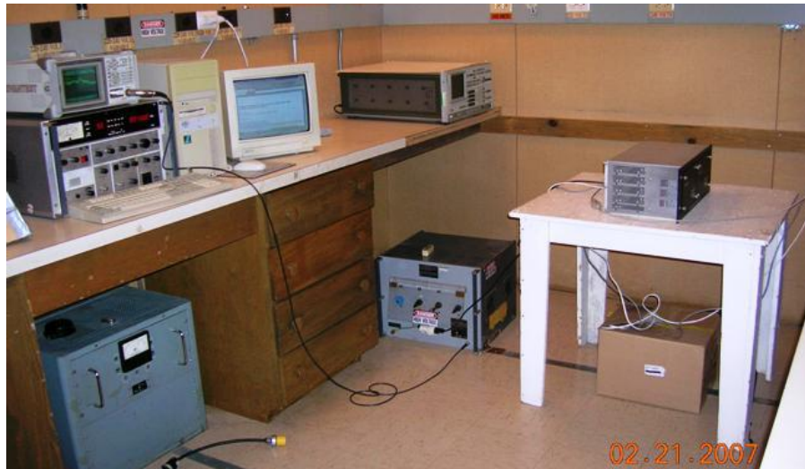
Figure 23 Picture taken to the set up of the conducted emissions measurements. Source: Author.
