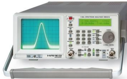
Figure 5 Example of a spectrum analyzer. Developed by Hameg, model HM5510
