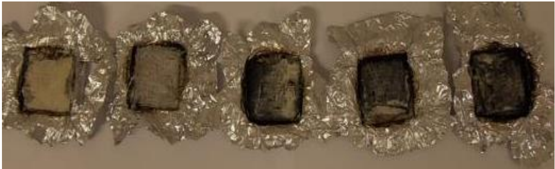
FIGURE 27. Composite residues after MLC. View from top. From left to right: FlaxPLA, FlaxPLA+NaOH, FlaxPLA+AS, FlaxPLA+APTES, FlaxPLA+NaOH+APTES
