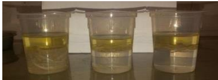
FIGURE 24. Hydrophobicity test oil/water. From left to right: FlaxPLA, FlaxPLA+APTES, FlaxPLA+NaOH+APTES
