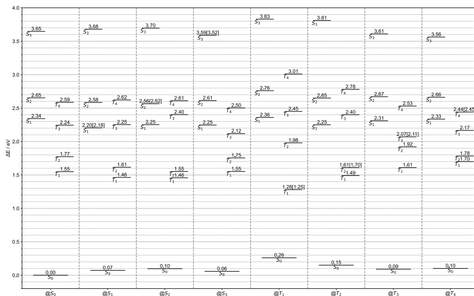
Figure 17. State energies (DFT, [eV]) calculated at the optimized geometries of the S 0 , S 1 , S 2 , S 3 , T 1 , T 2 , T 3 , T 4 states of methylpheophorbide a. All energies are set relative to the ground state energy at S 0 geometry and computed under TDA.
