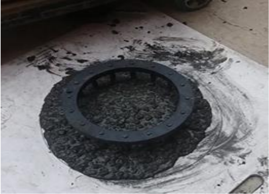
Figura 16. Ensayo slump test (slump flow, test-500) a/c=0.6 IS=40%.
