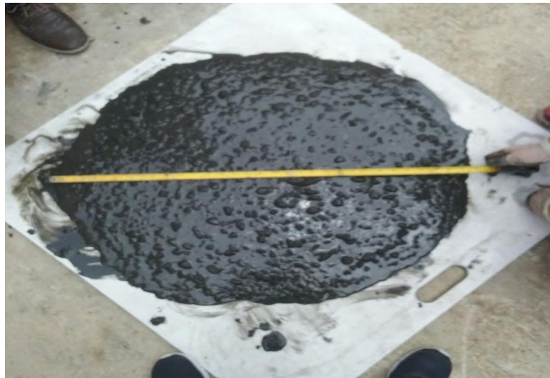
Figura 6 Ensayo slump test (slump flow, test-500) a/c=0.4 IS=0%.
