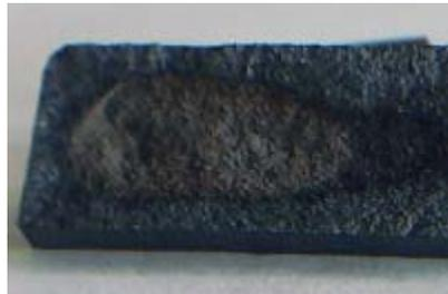
**FIG 7.1 PROBETA DE BRONCE CON CAPA DE OXIDO Y CENTRO SIN DESLUBRICAR**
