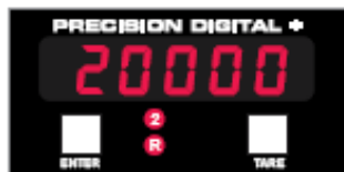
PD691 Alarm #2 Reset Point is adjusted to 20000.
