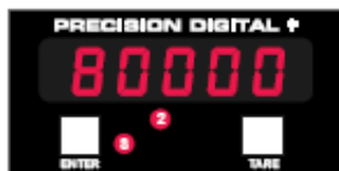
PD691 Alarm #2 Set Point is adjusted to 80000.
