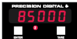
PD691 indicating that Alarm #2 is in alarm condition.
