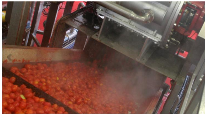
Figura 13. JBT. (n.d.). Calor por vapor. Retrieved December 6, 2019, from Saturno peeler website: https://www.jbtc.com/en/north-america/foodtech/products-and-solutions/products/choppers-corers-cutters-emulsifiers-and-peelers/peelers/saturno-peeler
