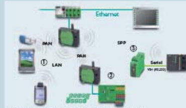
Operation as Bluetooth access point for connecting up to seven devices
