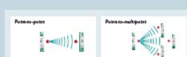
The unidirectional radio system offers traditional point-to-point connections and multiple receiver systems for signal splitting or signal multiplying.
