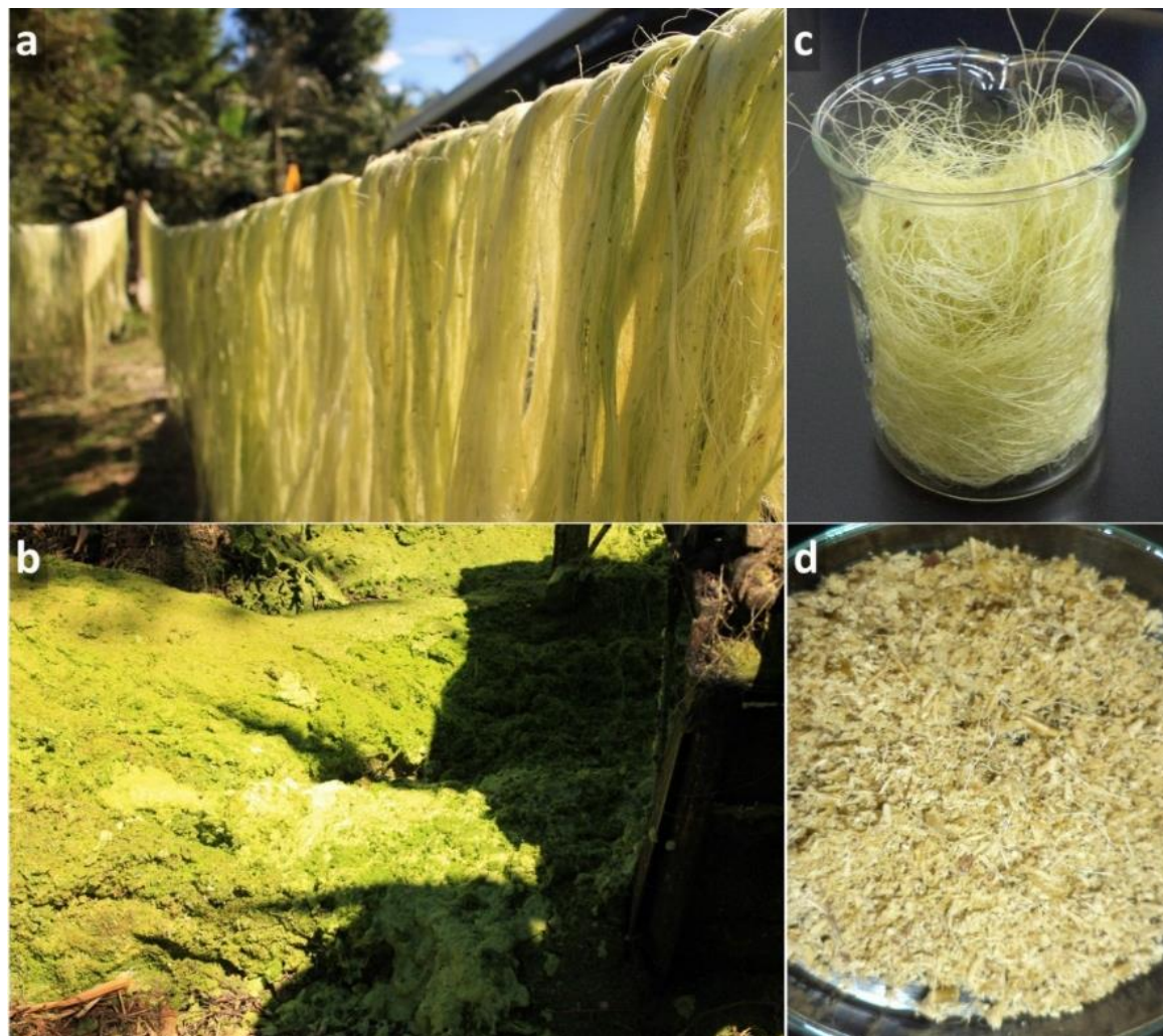
Figure 1. (a) Fique fibers, (b) Fique decortication residues, (c) Clean Fique tow, and (d) Clean Fique pulp
