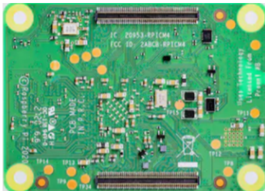
Figura 12. Raspberry Pi Compute Module 4.
