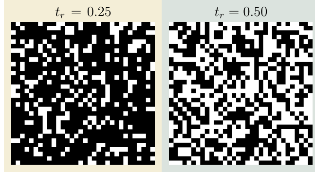
Figure 3. Sketch of boolean masks with transmittance t_r \in \{0.25, 0.50\} . The black and white pixels correspond to d \in \{0, 1\} coding elements, respectively.
