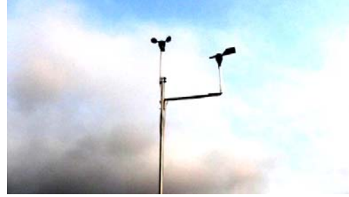
Figure 1. System's anemometer and wind vane
