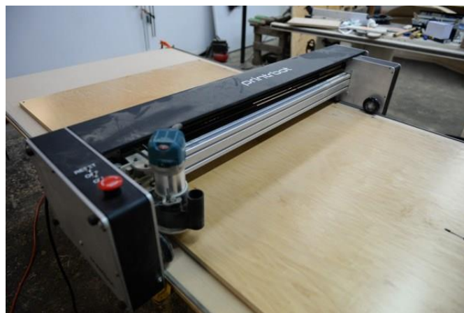
Figura 14. Printrbot Crawlbot. Nota: recuperado de “Review: Printrbot Crawlbot Changes Everything About Large CNC Routing”, de Loik, J., 24 de septiembre de 2015. Tomado de https://makezine.com/2015/09/24/printrbot-crawlbot-review/
