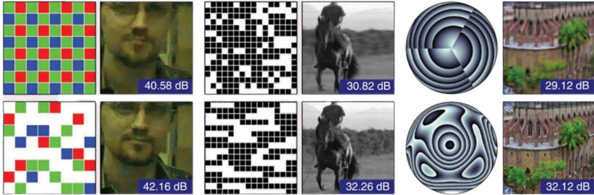
Figure 2.2. Multiple optimized, shown at the top, and not optimized, shown at the bottom, coding elements presented on [Arguello et al., 2023], where it is shown that the performance of the optimized coding elements increases compared with not optimized coding elements, where the first two columns show examples of amplitude encoding elements, while the last column shows an example for phase coding elements.
