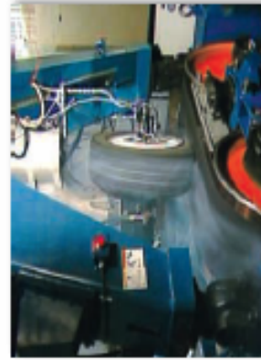
These Flat-Trac systems, with power and speed, generate accurate force and moment data that produce large lateral or longitudinal forces.
