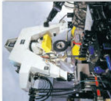
The FlatTrac LTA expands the testing envelope for dynamic tests on light truck, SUV and motor sport racing tires.
