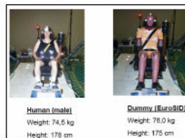
Figure 16. Test set up of the sled with dummy and volunteer
