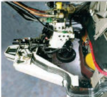
The FlatTrac CT provides a powerful torque drive for a broader range of dynamic force and moment testing.
