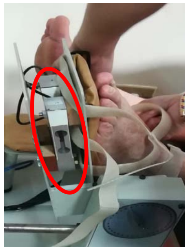
Figure 7. Detail view of load cells supported on two points
