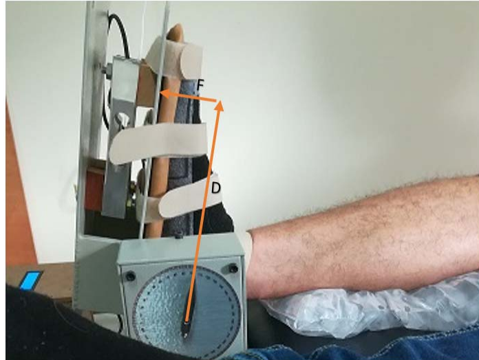
Figure 9. Distance for torque measurement and point of average force application
