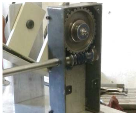
Figure 4. Detailed view of the worm-crown mechanism
