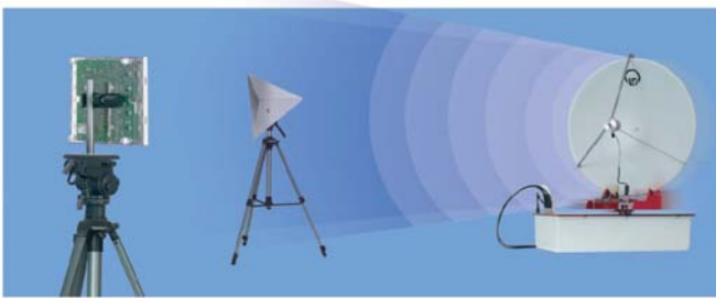
Experimental set-up for pulse sonar with corner reflector and transponder
