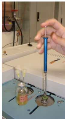
Fig. 12. Injection of the sample into the Gas Chromatograph (GC).
