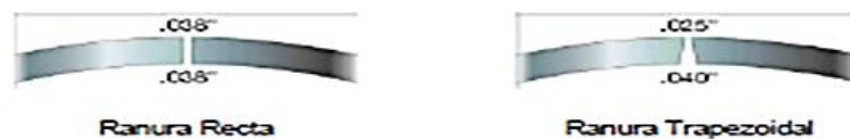
Figura 97. Ranura recta y ranura trapezoidal
