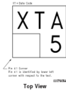
LM358TP micro SMD Marking Orientation
