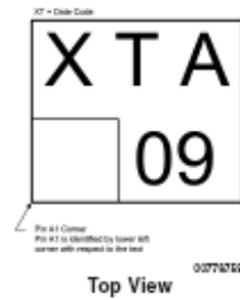
LM2904TP micro SMD Marking Orientation
