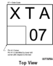
LM358TP micro SMD Marking Orientation
