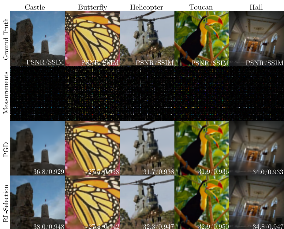
Figure 4.1. Visual reconstruction comparison for PGD and RL-Selection. Results obtained with CR=0.3 and noise level with \sigma = 0.02 for various standard test images, highlighting the preservation of textures in the RL-based approach.
